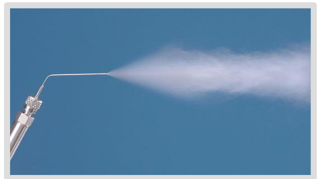
Figure 2. A microsprayer used for aerosol dosing directly into the lungs (Microsprayer® Aerosolizer Pulmonary Aerosol Kit for Mouse, Penn-Century Inc.; Wyndmoor, PA).
